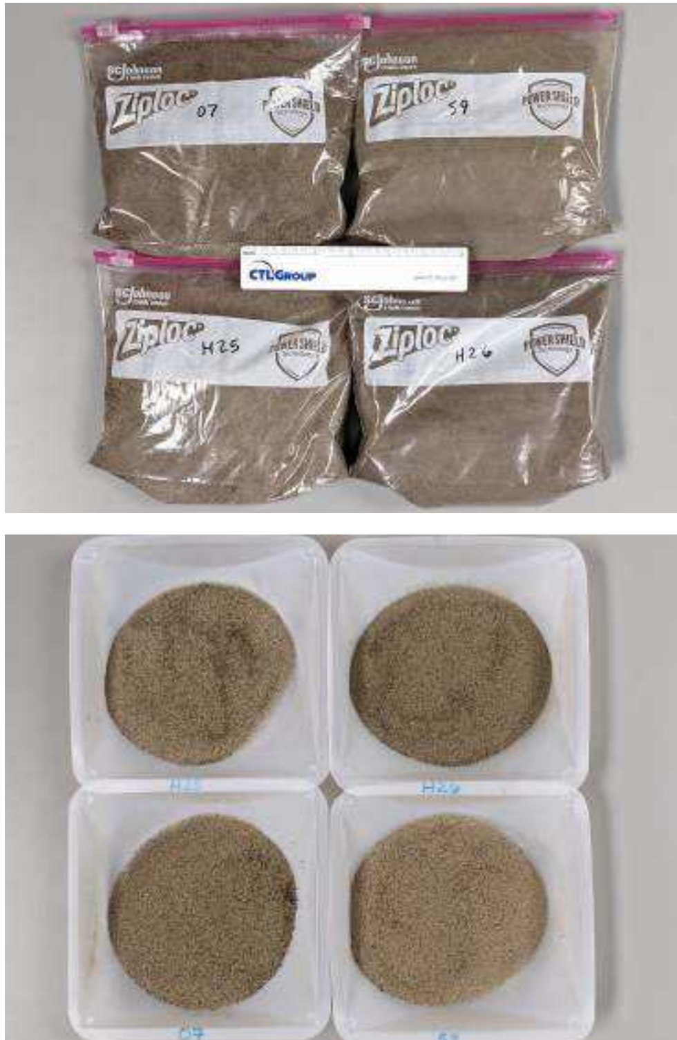
Fig. 1 Top photograph shows the samples received for examination. Bottom photograph shows the 35 to 38 gram test specimens.
