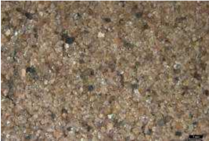
3a. Black CCR particles intermixed with predominantly quartz sand particles.
