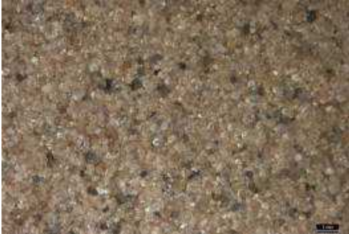
2a. Black CCR particles intermixed with predominantly quartz sand particles.
